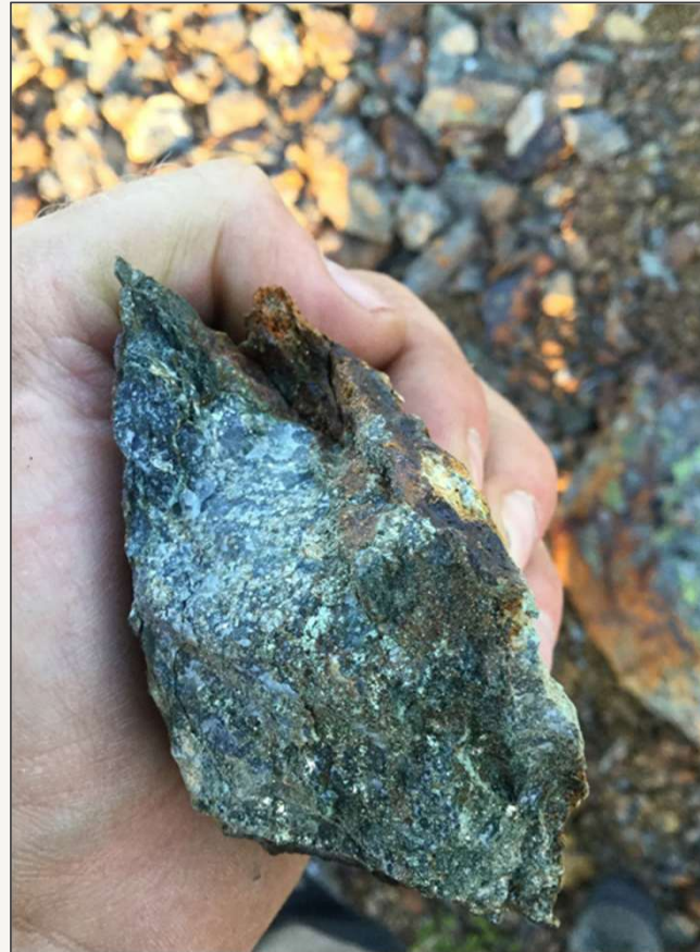
Dump samples from Malså area. Massive sulphide with quartz, pyrite, chalcopryrite.
